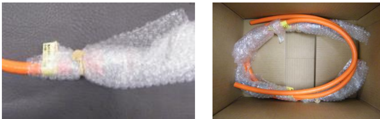
Picture 4: Eyelet connector covering/wrapping and placement in the box
