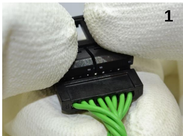
Recommended procedure for male housing hinged secondary lock engagement.
