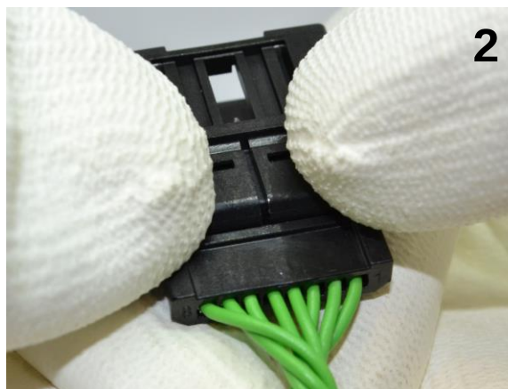
Recommended procedure for male housing hinged secondary lock engagement.
