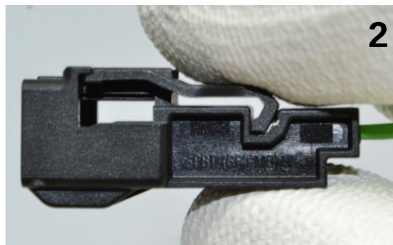
Housing hinged secondary lock in set position.
